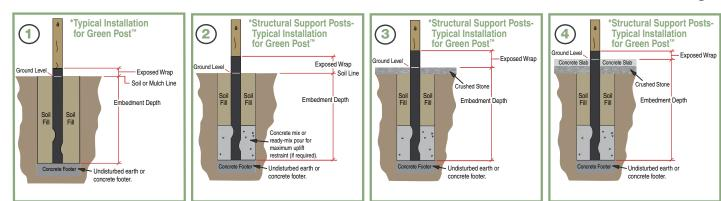
Uplift Restraint Notches are enlarged for illustration purposes.
