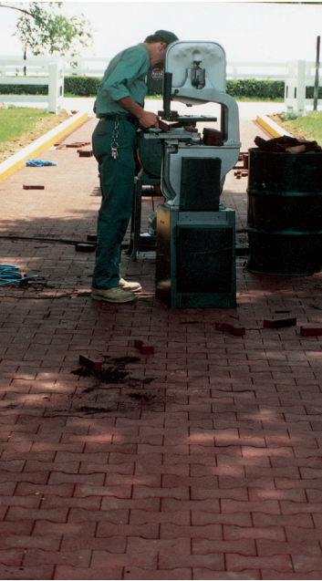
Pavesafe can easily be cut with a heavy duty band saw or a break-off-blade utility knife, pending the size of the project.
